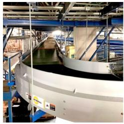
The overriding strategy of this project was to provide a costsensitive solution for improved performance and reliability of the systems in these two facilities. Specifically, to include replacement of belt-curves. This tactic required that our engineering team utilize existing structural and electrical infrastructure, as a cost-saving measure.
